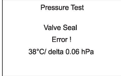
Check the connection between the valve and head, especially cable connector. Other reason can be faulty coil in the valve or faulty valve.
