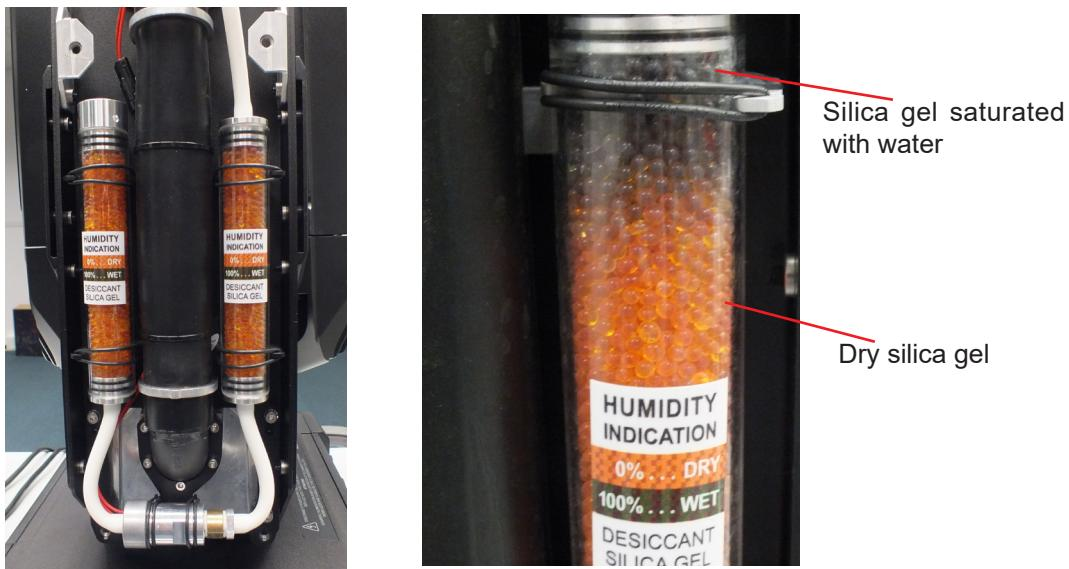
State of desiccants in the fixture arm can be checked:
