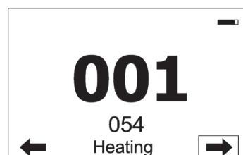
The fixture is waiting for reaching operating temperature of the fixture inside (inside temperature is below 0°C).
