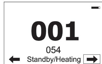
The fixture is in standby mode and inside of the fixture is heated (ambient temperature is below 0°C).
